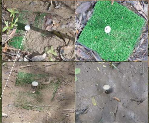
Due to sediment transport and deposition, the open water area of Searsville Reservoir is now much reduced from its historical extent (approximated by the blue line). Sediment traps (above) placed in areas of the Corte Madera Creek floodplain (white dots) record the amount of deposition when the creek overtops its banks. The orange line is the JRB boundary.
