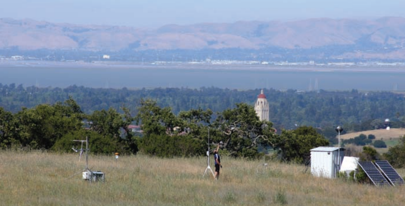
Left: Sensor arrays and photovoltaic power make up the eddy covariance station, which calculates carbon uptake and loss by the ecosystem based on relationships between air turbulence and CO 2 concentration.
