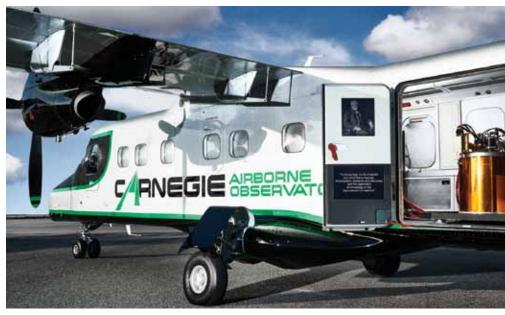
Inside a twin turboprop plane, the CAO houses two types of imaging spectrometers and a dual-laser, waveform light detection and ranging (wLIDAR) scanner. These three instruments are used in combination to map vegetation chemistry, biomass, structure, and stress.
